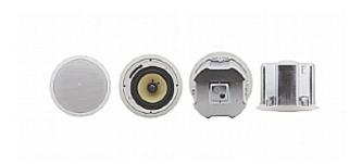
The Yarden 8–C Closed–back High Performance Ceiling Speaker features a Kevlar(R) woofer, 2nd level cross–over design and multi–tap power transformer for selecting  $8\Omega$  (bypassing the transformer) or 70V/100V power settings that are suitable for an array installation.
