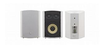
The Yarden 6-OD High Performance On-wall Stereo Speaker features a Kevlar (R) woofer, dual pivoting titanium tweeters, 2nd level cross-over design and multi-tap power transformer for selecting  $8\Omega$  (bypassing the transformer) or 70V/100V power settings that are suitable for an array installation.
