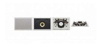
The Yarden 6-ID High Performance In-wall Stereo Speaker features a Kevlar(R) woofer, dual pivoting titanium tweeters, speech mode to improve intelligibility, 2nd level cross-over design and multi-tap power transformer for selecting  $8\Omega$  (bypassing the transformer) or 70V/100V power settings that are suitable for an array installation.
