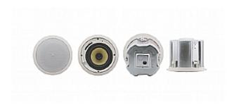
The Yarden 6–C Closed-back Compact High Performance Ceiling Speaker features a Kevlar(R) woofer, 2nd level cross-over design and multi-tap power transformer for selecting  $8\Omega$  (bypassing the transformer) or 70V/100V power settings that are suitable for an array installation.
