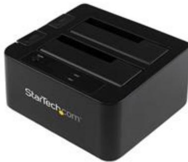
The SDOCK2U33EB Dual 2.5/3.5" SATA hard drive docking station lets you dock and swap hard drives from your desktop or laptop computer simultaneously using a single eSATA or USB port.
