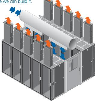
Typical hot aisle/cold aisle configuration with hot air vent to the plenum via a Chimney Top (ECTOPCHIM), **p. 11**. Also shown is the Cold Aisle Containment System (EC45U48WCD), **p. 11**.
