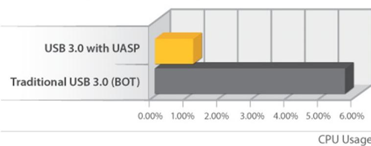
Test results were obtained using an Intel® Ivy Bridge system, StarTech.com add-on USB 3.0 cards, a UASP-enabled StarTech.com enclosure, and a SATA III solid state drive.
