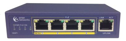
between full and half duplex modes, so any port can connect to a Fast Ethernet or Ethernet network. The ports also support Auto MDIX, allowing the automatic detection of a straight through or cross-over cable, this feature reduces support problems commonly caused by incorrect cable usage.
