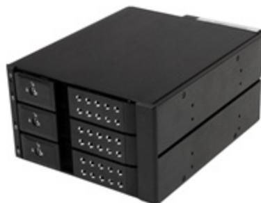
The HSB3SATASBA Removable 3-drive backplane lets you quickly install and hot-swap 3.5" drives from the front of your computer, by turning two 5.25" bays into a hot-swappable interface for you to connect up to three 3.5" SATA or SAS hard drives (HDD).
