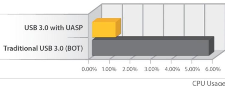
Testing results were obtained using an Intel® Ivy Bridge system, a UASP-enabled StarTech.com Enclosure, and a SATA III solid state drive.
