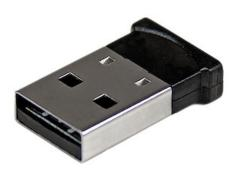
The USBBT1EDR4 USB to Class 1 Mini Bluetooth Dongle lets you add Bluetooth wireless capabilities to a laptop or desktop computer through USB, with support for transfer distances of up to 50m (165ft).
