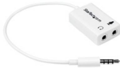
The MUYHSMFFADW Headphone/Microphone Splitter features one 4-pole (4-pin) 3.5mm male (TRRS) and two 3-pole (3-pin) 3.5mm (TRS) female connectors, enabling you to add a mono microphone input, as well as a stereo output to your PC or Laptop, through a single 3.5mm audio port.
