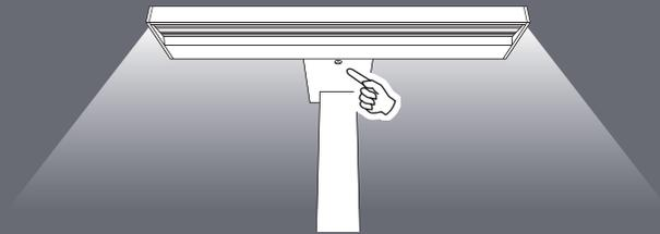
Pushbutton on each luminaire for personal task light control.
