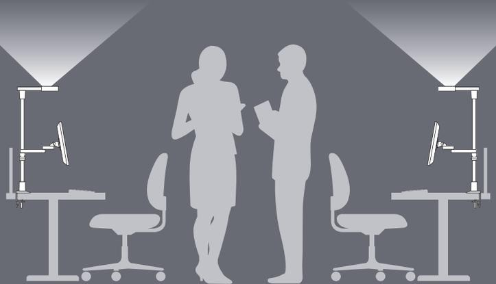
Uplights connect to room controls and provide glare-free, indirect ambient light for collaboration and general office tasks.
