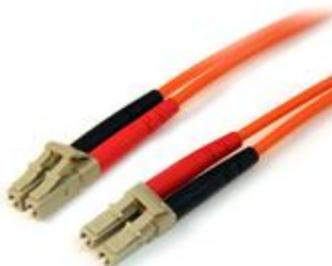
The 50FIBLCLC30 30m LSZH LC to LC Fiber Cable features 50/125 micron fiber for high-speed, high bandwidth data transmissions over Gigabit Ethernet and Fiber Channel networks, with support for duplex multimode applications.
