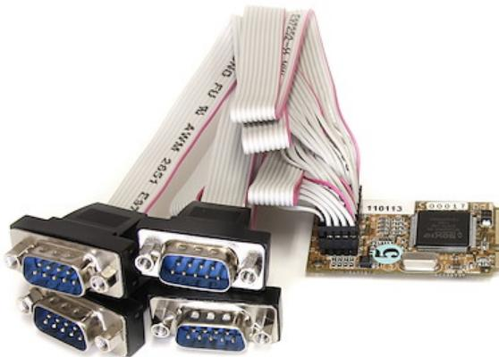
The MPEX4S552 4-Port RS232 Mini PCI Express Serial Card (16650 UART) turns a mini-PCIe slot into four RS232 (DB9) serial ports with data rates up to 921.6 Kbps - a cost-saving solution for adding serial support to embedded systems missing the functionality.
