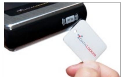
Unlock with RFID token (optional RFID 2 factor authentication)
