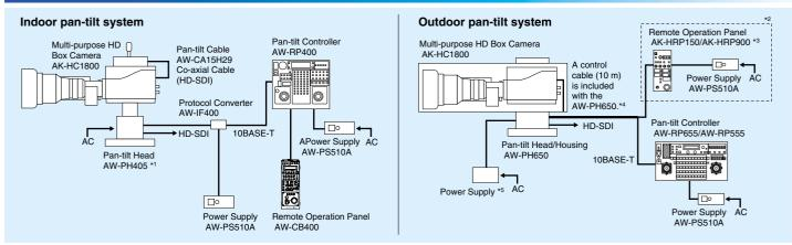
\*1 Up to five Pan-tilt Head for one Pan-tilt Controller can be used. \*2 AW-RP655 can control an AK-HC1800 without AK-HRP150 or AK-HRP900. \*3 AK-HRP900 is not available in PAL (50 Hz) area. (Please ask to local Panasonic sales company for detail information.) \*4 An accessory cable may be used for the AK-HRP900. \*5 An AW-PH650 includes a power supply.
