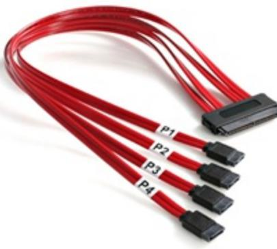
The SAS84S450 SFF-8484 to 4x SATA SAS cable features one 32-pin receptacle (SFF-8484) which fans out to four SATA 7-pin receptacles, providing a reliable solution for connecting up to four SATA HDDs to a SAS controller or backplane.
