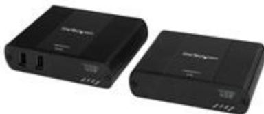
The USB2002EXT2 2-Port USB Extender lets you extend USB 2.0 devices over Cat 5 or better Ethernet cable at distances of up to 330ft (100m). A local transmitter power adapter provides up to 500 mA of power per port with no power adapter required at the remote end, letting you access and power almost any USB 2.0 device in locations where a power outlet may be unavailable.
