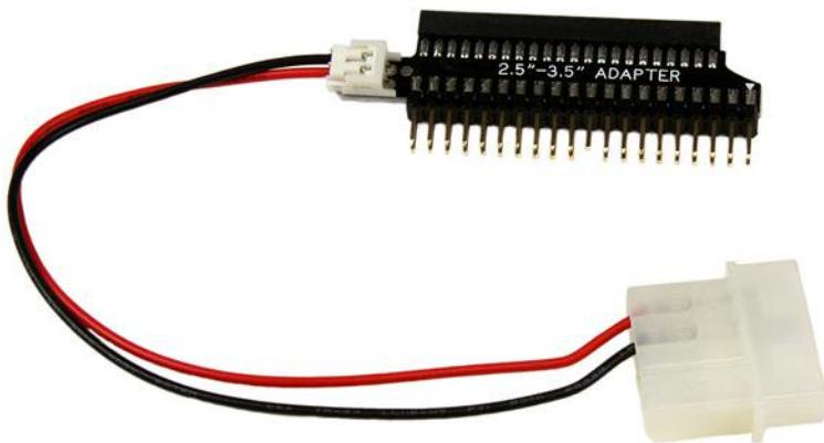
This 2.5in to 3.5in IDE Hard Drive Adapter cable provides a 44-pin female IDE connector and a 40-pin male IDE connector as well as an LP4 power supply connection, allowing you to connect a 2.5in IDE laptop hard drive to a desktop computer.
