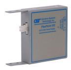
Designed for telecommunications and IT applications such as campuses and phone centers that use DC power as a primary power source, the FlexPoint DC Converter allows any FlexPoint media converter to be powered from an 18 to 60VDC power source. Not for use in the FlexPoint 5-Module Rack-Mount Shelf.
