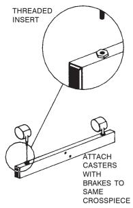
■ Using the wrench supplied, firmly screw (N) Casters with Brakes and (O) Casters without Brakes into threaded inserts found in (O) Lower Crosspieces. Note: Install both casters with brake into same crosspiece.
