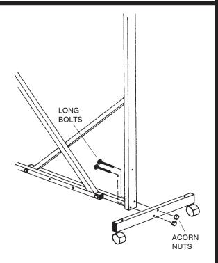
Fasten © Lower Crosspiece, with casters installed, to L-frame as shown, using two Long Bolts and two Acorn Nuts. Tighten with wrench. Repeat for opposite side.
