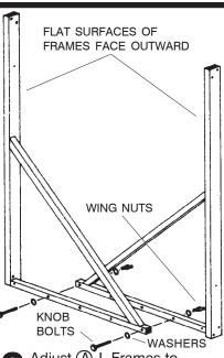
Adjust (A) L-Frames to length of hanger to be used. Secure using two (Q) Knob Bolts, four (R) Washers, and two (P) Wing Nuts as shown. Note: In all cases, hole at END of each L-frame must be used.
