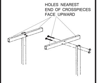
Install a ① Top Panel in the position shown, using three ⑥ Short Screws. Next, fasten two ⑥ Plastic Spacers to ends of crosspiece using ① Long Screws. Cover spacers and screws with ① Black Plastic Caps.
