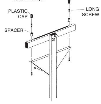
Peel paper from a S Black Plastic Strip. Position it, with the sticky side down, along the INSIDE top edge of the upper crosspiece as shown, and press down. Note: strip must be even with edge for unit to work properly. Repeat for other side.
