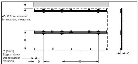
"D" = 1/2 of Display Width, Side of video wall to the center of first wall plate.
