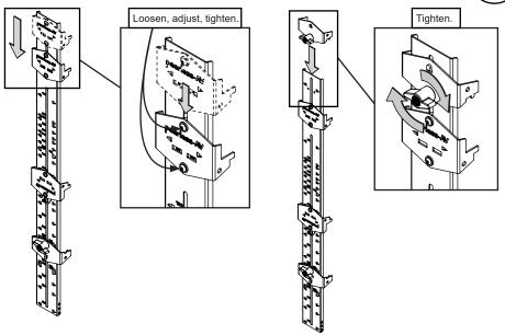
Install remaining extrusions using the spacers. Clamp the upper spacer jaw assembly to an uninstalled extrusion assembly. Clamp the bottom spacer jaw assembly to the installed extrusion. Vertically align extrusions with a laser. Drill mounting holes into supporting surface and install wall plates to the wall.
