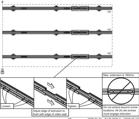
Set the laser level so that it is parallel to the mounting surface (wall). Measure from wall to laser in various locations and find the wall's high point. Mount the laser target at the location that is near the wall's high point and closest wall plate. Adjust the extrusion out slightly from the wall, tighten wall plate screws and mark laser line on the target. Move the target to the remaining wall plates, adjusting depth until the laser is on the line, tightening the screws as you go.
