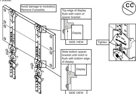
Remove display. Return top spacer bracket to the 80mm position. Replace top clamp onto assembly.
