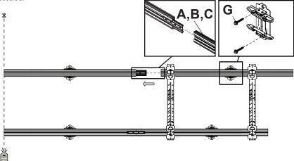
Once the entire row is installed, compare the length of the extrusion to width of the video wall. If the extrusion is shorter, use the expansion joint to extend the overall length of the extrusion so that it is flush with the video wall. The expansion joint can be extended up to 160mm.
