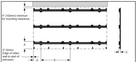
"D" = 1/2 of Display Width, Side of video wall to the center of first wall plate.
