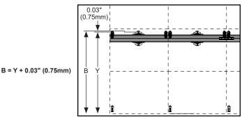
For even number of rows, start with extrusion at second row of displays from the bottom.
