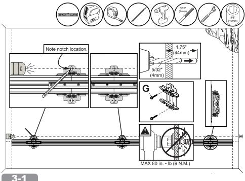
Determine the combined height of TWO displays being mounted and locate the same dimension on the front of spacer. If height is above 686mm, attach spacer extension. If height is not listed on the spacer, use measurement of the combined height of TWO displays to set custom spacing.
