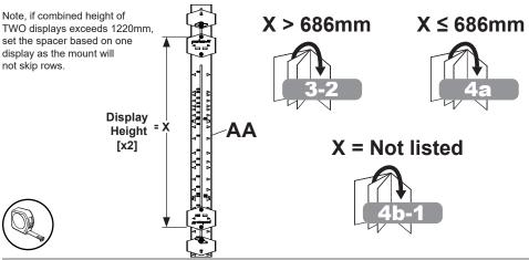
Add the extension when "X" measurement (step 3) is taller than 686mm. Detach lower fixed jaw and clamp bracket from main spacer assembly and reattach to the extension.
