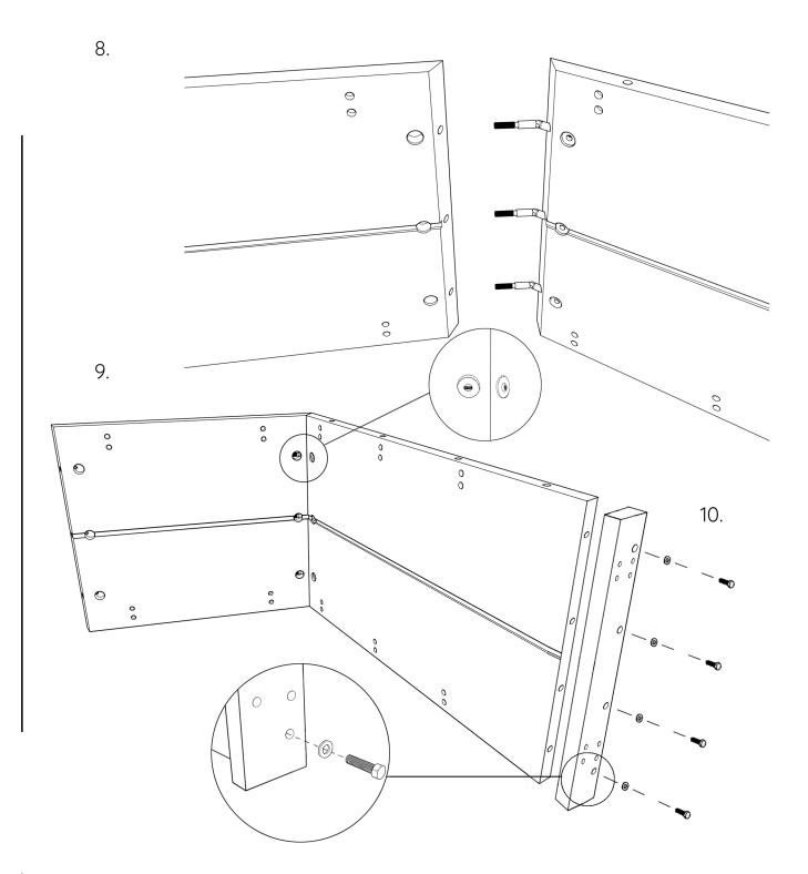
11. Tighten both sets of screwheads alternately until the side and roof are in perfect alignment.
