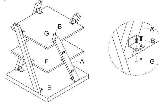
(4) Use the Screw (D) to install the L Bracket (C) to the Top (E).
