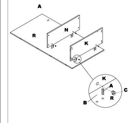
Insert Wood Dowels (A) into Back Panel (R), Bottom (K), Fixed Shelf (N), and Toe Kick (L). Insert Cams (C) into Back Panel (R) Fixed Shelf (N), and Bottom (K). Install Cam Posts (B) into threaded inserts in Right Side Panel (Q). Press Toe Kick (L) to Bottom (K). Attach Right Side Panel (Q) to Back Panel (R), Fixed Shelf (N), and Bottom (K) by turning Cams (C).
