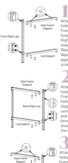
Attach Leg Support (no holes in flange) and Side Frame Support (with holes in flange) to Front Right Leg using 4 Pan Head Screws and 4 Washers (ensuring Washers are snug against the head of the screws).
