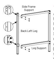
Attach Leg Support (no holes in flange) and Side Frame Support (with holes in flange) to Front Left Leg using 4 Pan Head Screws and 4 Washers (ensuring Washers are snug against the head of the screws).
