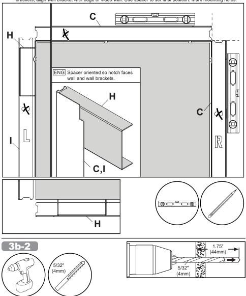
ENG Drill mounting holes into supporting surface (1.75" (44mm) minimum depth required).
