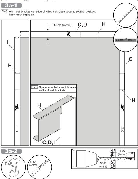
ENG Drill mounting holes into supporting surface (1.75" (44mm) minimum depth required).
