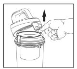
Pull dust cup latch to lift up dust cup lid.
