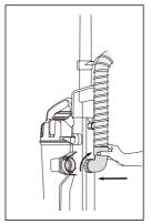
Insert bent end of hose into opening at back of dust cup. Twist hose clockwise to lock.
