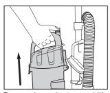
Press release button and lift off dust cup.
