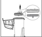
Lift out foam filter and shake off dust. Rinse foam filter and dry THOROUGHLY.
