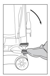
Step on handle release to lower handle into position for vacuuming floors.
