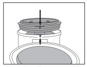
Align tab on filter screen with slot on back of dust cup and drop into position.
