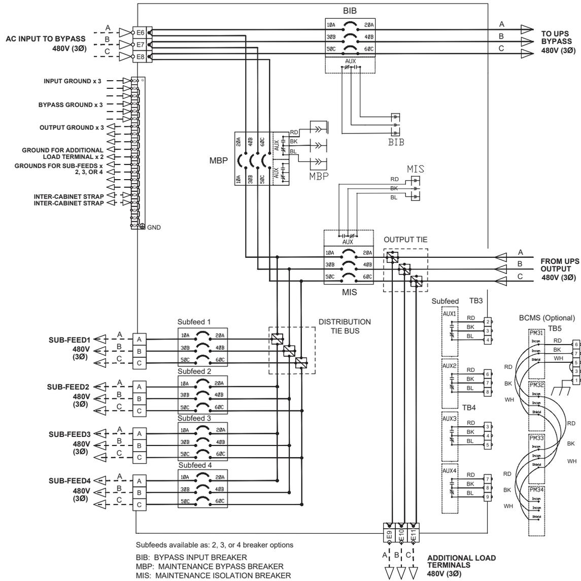
**Figure 32. Eaton 93PM 400 kW IAC-BD Breaker Auxiliary Contact Schematic**
