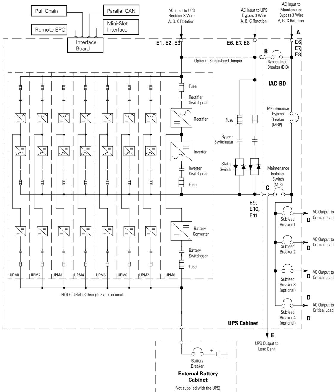
Figure 31. Eaton 93PM 400 kW IAC-BD Schematic – Three Breaker Maintenance Bypass
