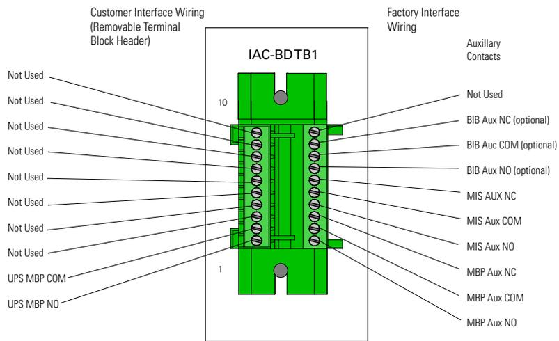
NOTE 1: The removable terminal block header faces up when installed. The terminal block is shown rotated 90 degrees counterclockwise for clarity.
