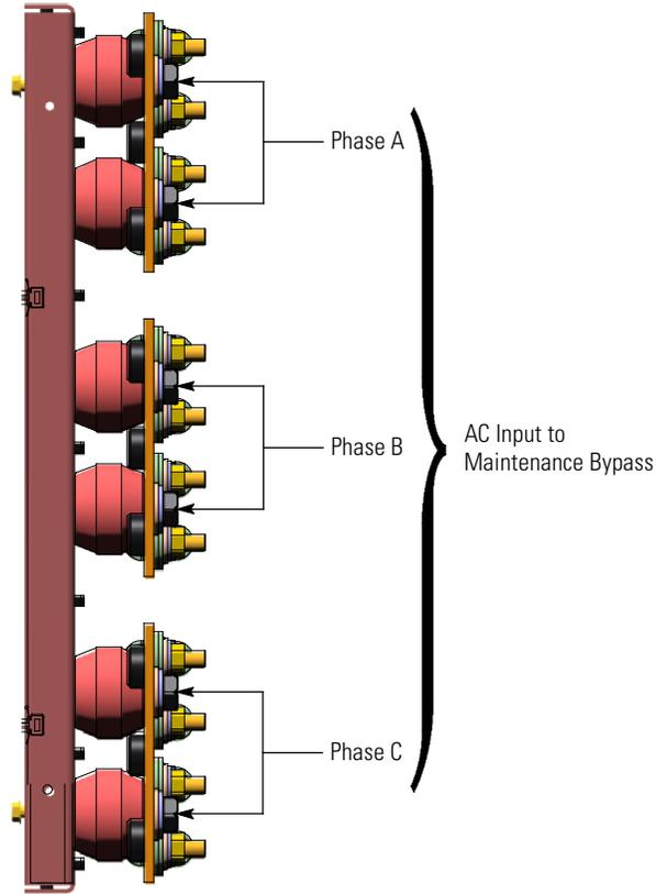
**Figure 17. 93PM IAC-BD Subfeed Breaker without PM3 Module Terminal Detail**
