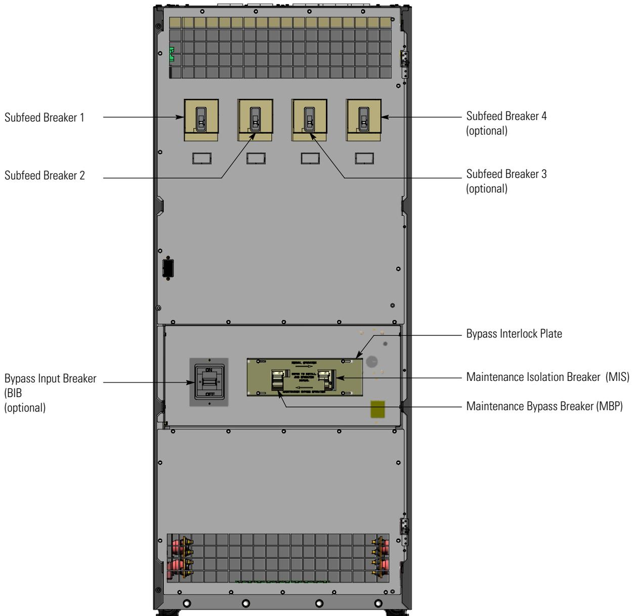
Figure 35. 93PM IAC-BD Breakers – Trapped Key Interlock
