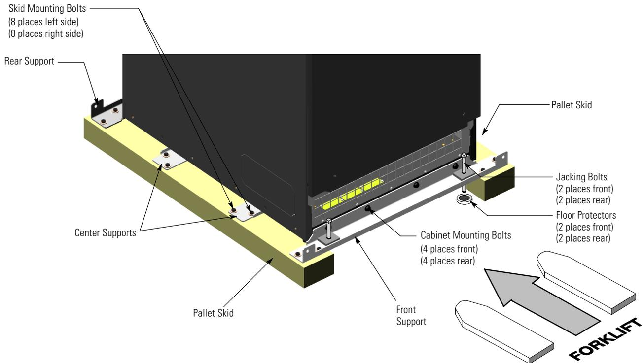
4. Loosen, but do not remove, the skid mounting bolts holding the left, right, front, rear, and two center supports to the pallet skids (see [Figure 10](#)). DO NOT loosen or remove the cabinet mounting bolts or the cabinet support bolts.
