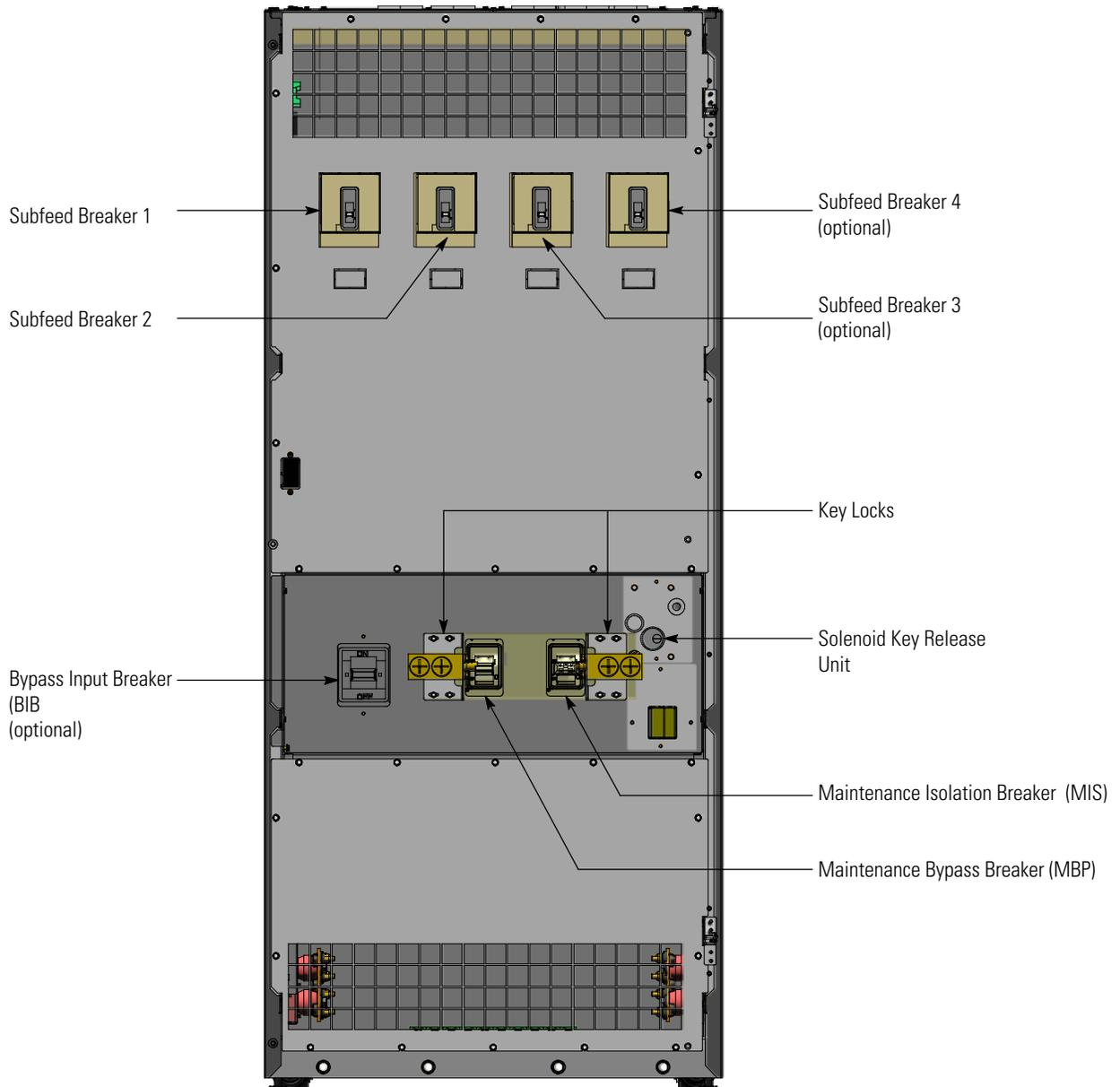
**Figure 36. 93PM IAC-BD – Trapped Key Interlock Detail**
