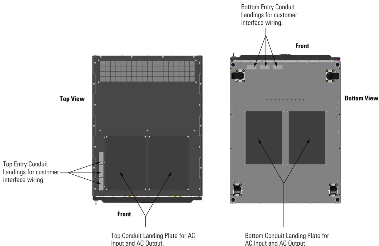
NOTE: Remove panels to drill or punch conduit holes
