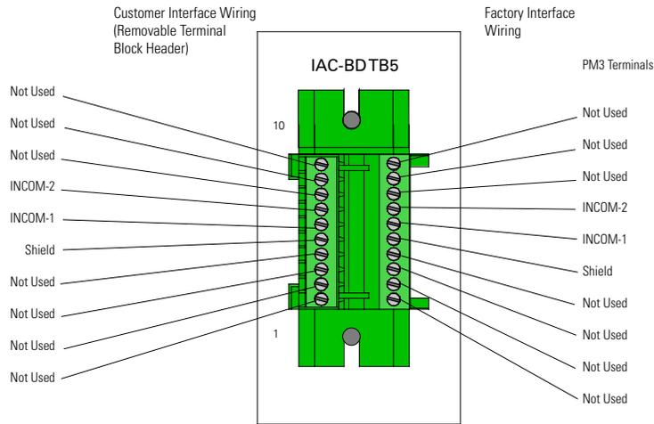
NOTE 1: The removable terminal block header faces up when installed. The terminal block is shown rotated 90 degrees counterclockwise for clarity.
