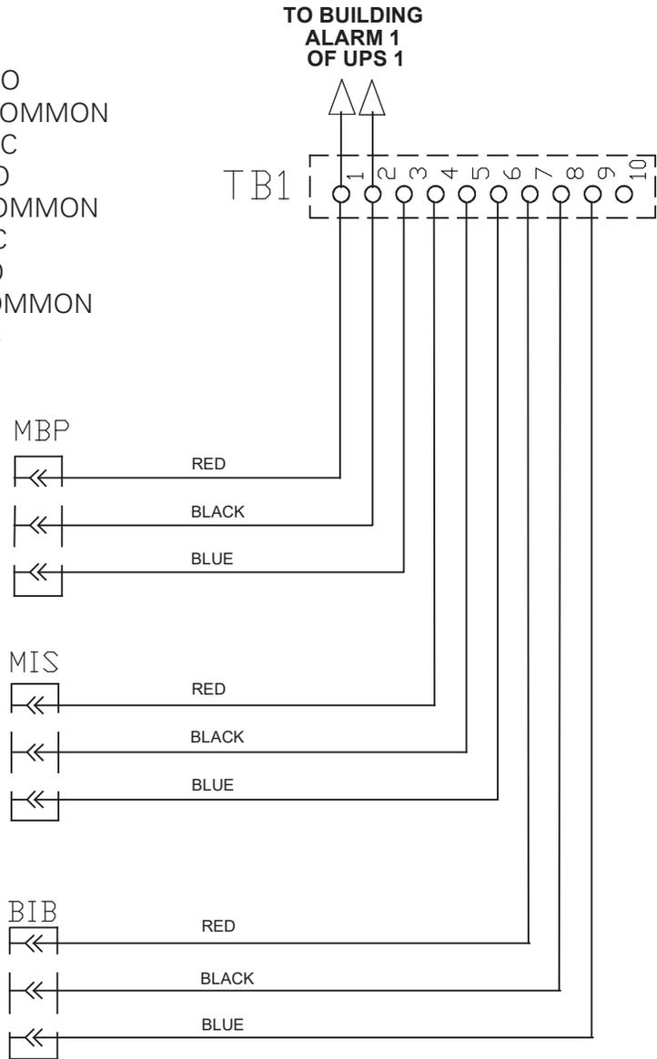
**Figure 33. Eaton 93PM 400 kW IAC-BD Kirk Key and Solenoid Key Release Unit (SKRU) Schematic**
