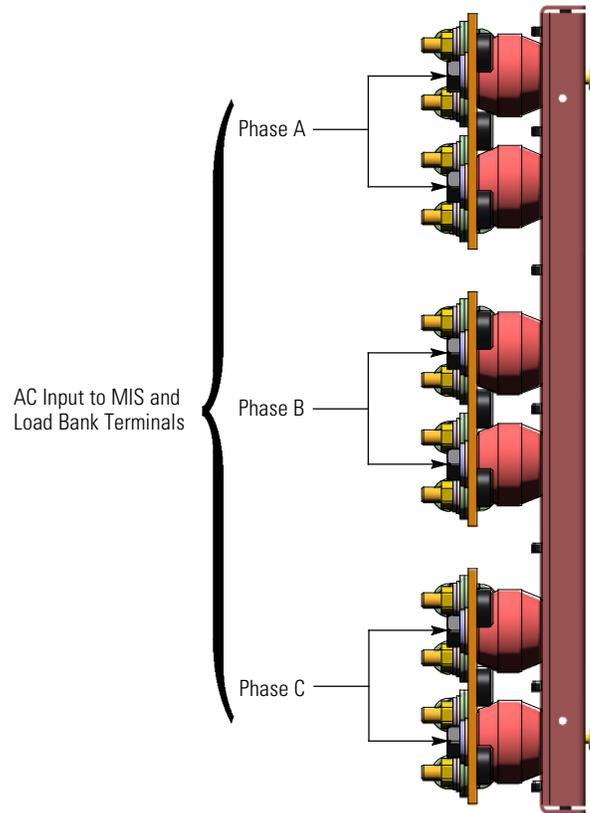
Figure 16. 93PM IAC-BD Maintenance Bypass Input Terminal Detail
