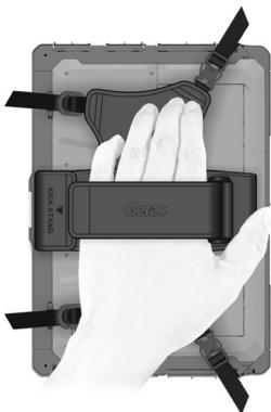
The hand grip is rotatable. The tightness can be adjusted.
