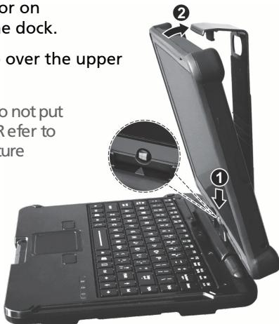
4. Firmly press down the clamp to ensure that the clamp fully locks F110 in place.
