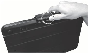
3. Align the Windows logo button on F110 with the triangle marking on the dock and attach F110's lower side at an angle (as shown by ①). This should match the docking connector on F110 with the connector pins on the dock.
