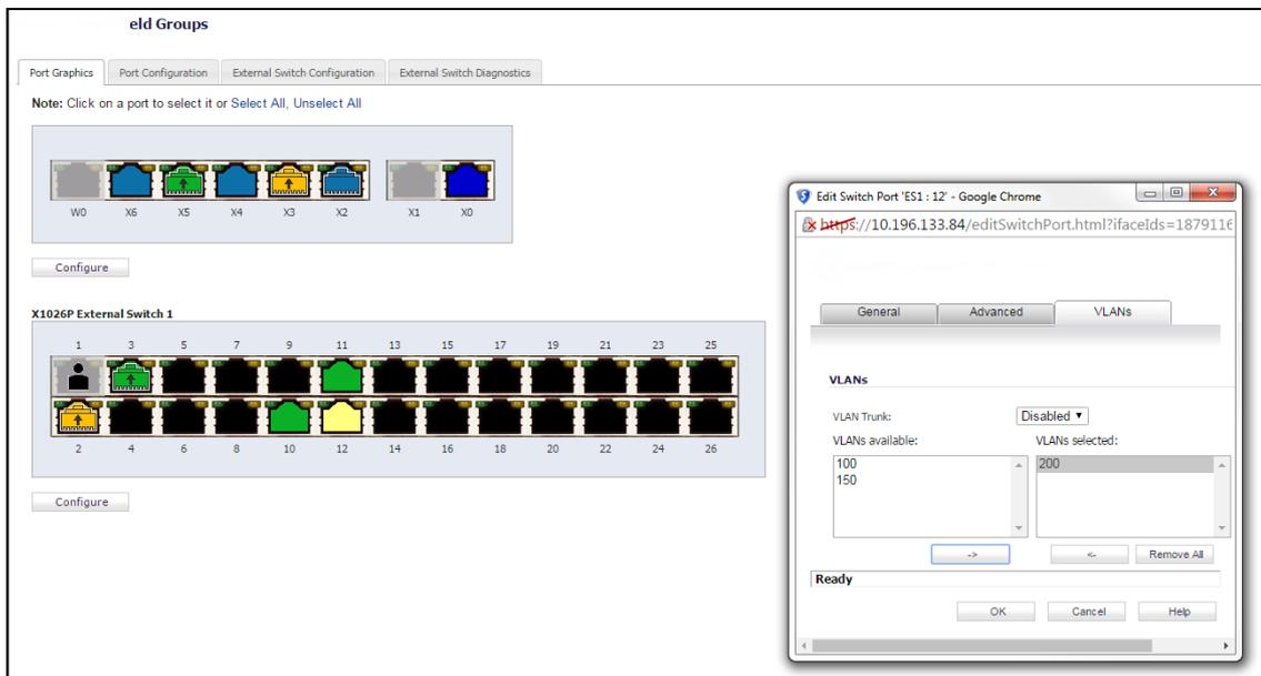
With this configuration, port 3 on the extended switch carries tagged traffic for VLANs 100,150, and 200 and untagged traffic for IDV VLAN 6. Port 10 is a trunk port carrying tagged traffic for VLAN 100, Port 11 is a trunk port carrying tagged traffic for VLAN 150, and Port 12 is an access port carrying untagged traffic for VLAN 200. Ports 10, 11, and 12 are portshielded to X5 through the dedicated link between X5 and port 2.
