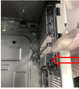
Figure43 Loose the 2 screws to remove the front handle from chassis
