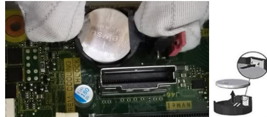
Figure22 Remove the battery from the MB
