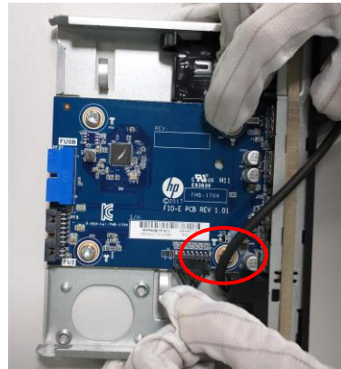
Figure34 Release the front panel mount cable by push out 2 pins fixed black side in switch card tray.
