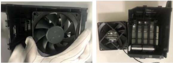
Figure27 Press the 2 latch to Separate the fan from front fan housing
