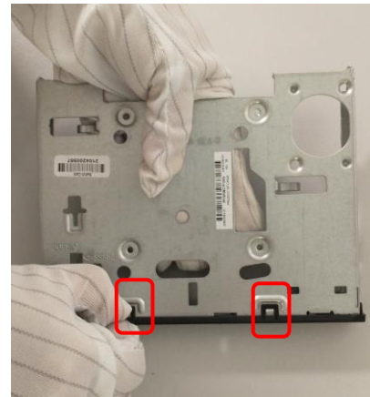
Figure38 Loosen the 2pcs bottom side hooks of switch card panel
