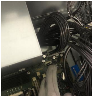
Figure7 Disconnect the cooler cable from MB and remove the cooler.
