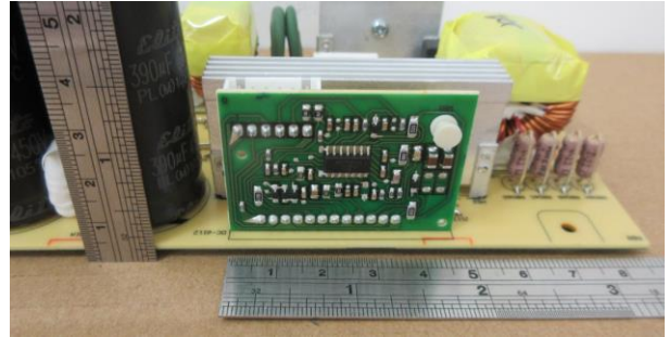
Figure50 Identity PCBA > 10 cm 2 for further treatment (DC-6112 board: 14.72 cm 2 ).
