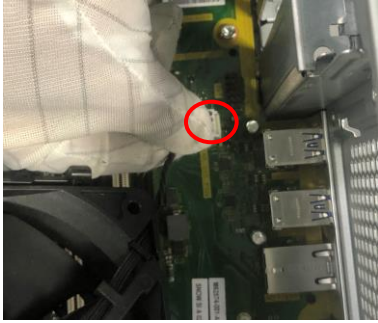
Figure17 Disconnect rear system fan cable from MB and remove the fan.
