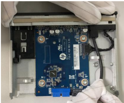
Figure31 Release the front panel mount cable from clip
