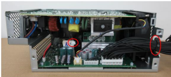
Figure47 Use tool to remove the cable tie.
