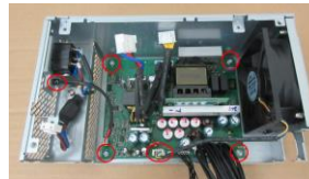
Figure52 Remove the LED cable from CASE by hand-pulling. Disconnect fan connector from PCBA. Use tool to unscrew four screws to loosen Main board. Remove Main board.
