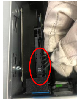
Figure12 Disconnect the HDD SATA cable from HDD
