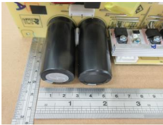
Figure51 Identity electrolyte capacitor > 2.5 cm for further treatment (Length: 5 cm).
