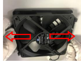
Figure18 Press the 4 latches to separate the fan guard from rear system fan
