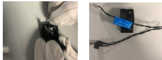
Figure20 Separate interlock holder from cable
