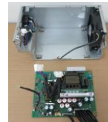
Figure52 Remove the LED cable from CASE by hand-pulling. Disconnect fan connector from PCBA. Use tool to unscrew four screws to loosen Main board. Remove Main board.
