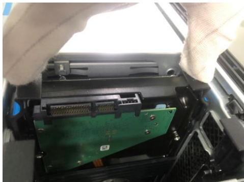
Figure15 Press the HDD's latch on HDD tray, and remove the HDD tray from HDD cage
