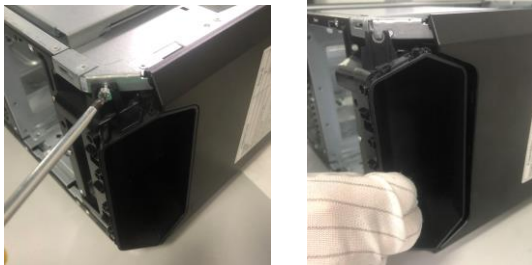
Figure43 Loose the 2 screws to remove the front handle from chassis
