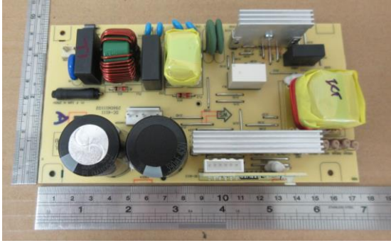
Figure51 Identity electrolyte capacitor > 2.5 cm for further treatment (Length: 5 cm).
