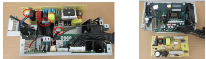
Figure48 Disconnect AC inlet connector and CN602A, CN601B cable connector from PCBA .Remove EMI board.
