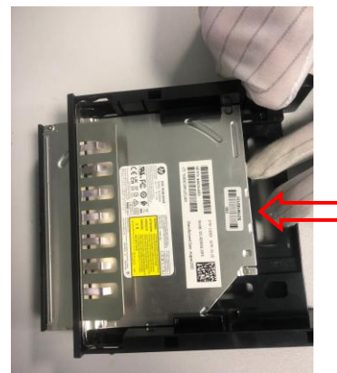
Figure40 Remove the DVD from chassis
