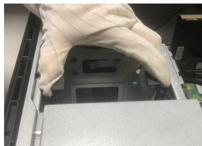
Figure6 Press the HDD's latch on HDD tray, and remove the HDD tray from HDD cage
