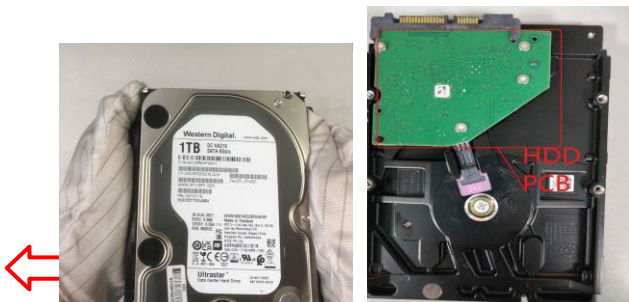
Figure5 Remove the HDD from HDD tray. See below HDD PCB area >10 sq cm.
