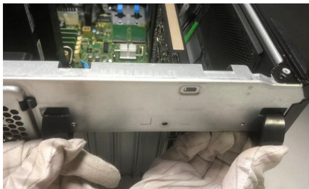
Figure9 Loose the PCIE retainer.
