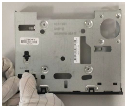
Figure42 Remove the SD card reader carrier.
