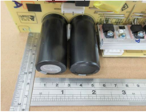
Figure53 Identity electrolyte capacitor > 2.5 cm for further treatment (Length: 5 cm).
