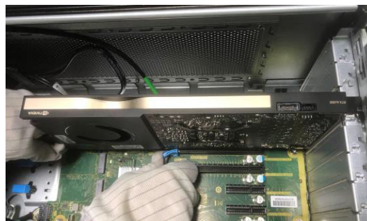
Figure10 Remove the graphic card from MB.
