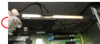
Figure7 Disconnect the cooler cable.
