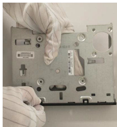
Figure44 Loosen the 2pcs bottom side hooks of switch card panel.
