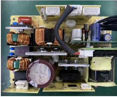
Figure39 Identity PCBA > 10 cm 2 for further treatment (main board: 19.795 cm 2 ).
