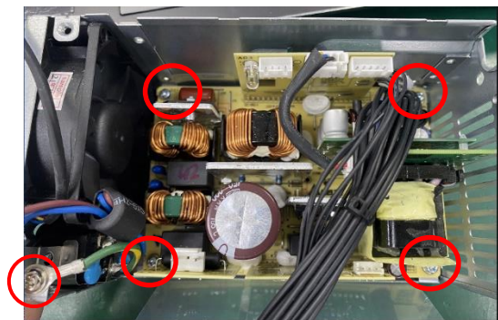
Figure33 Remove FG screw and PCB screw.
