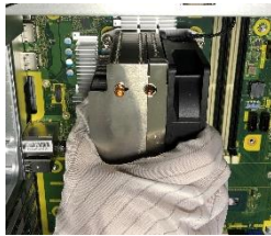
Figure23 Rotate the handle and open it up.
