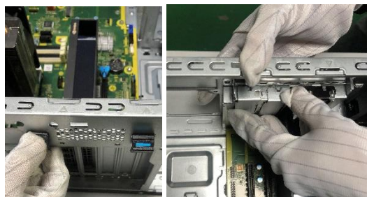
Figure15 Remove the PCI slot covers (x2) from chassis.
