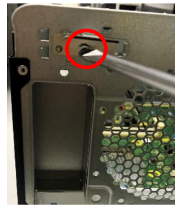
Figure28 Use Philip #0 screwdriver to loosen the screws of MB from board and remove the motherboard from chassis.
