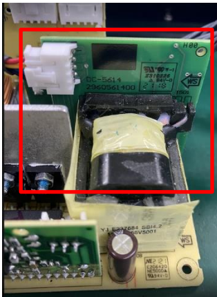
Figure41 Identity PCBA > 10 cm 2 for further treatment (main board: 26.956 cm 2 ).
