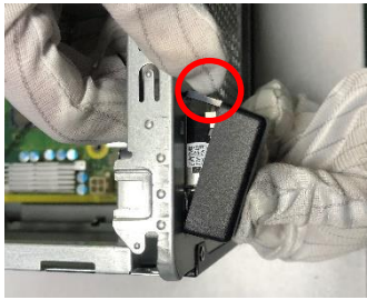
Figure25 Press the button and remove antenna cover.
