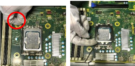
Figure23 Rotate the handle and open it up.
