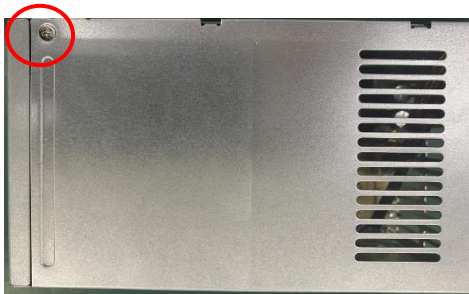
Figure29 Remove screw for case top.
