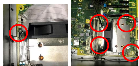
Figure20 Disconnect the cable and use Philip #0 screwdriver to loosen the screws.
