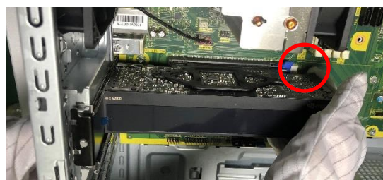
Figure16 Press the button and remove the graphic card from Motherboard. See below GFX PCB >10 sq cm.
