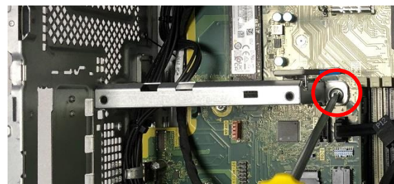
Figure6 Use Philip #0 screwdriver to remove the screws.
