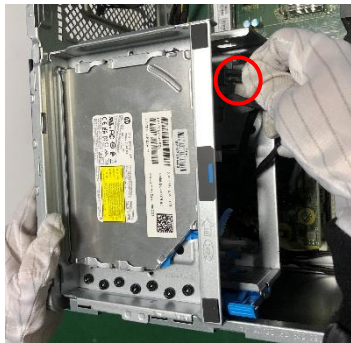
Figure5 Press the button and remove the ODD cage.
