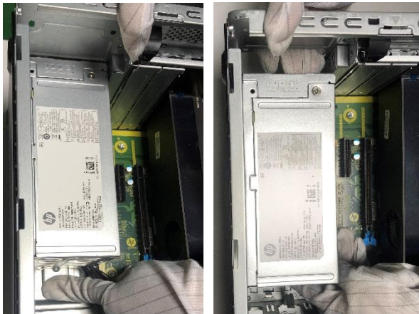
Figure14 Press the PSU's latch on chassis and remove the PSU from chassis.
