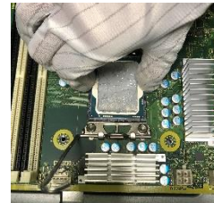
Figure24 Remove the CPU from motherboard.
