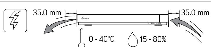
Covering the ventilation opening can result in overheating and system instability.
