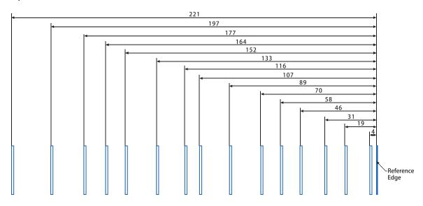
Rib pattern for Lexmark C4150, C4342, C4352, CS720, CS725, CS727, CS728, CS730, CS735, CX725, CX727, CX730, CX735, XC4140, XC4150, XC4342, XC4352
