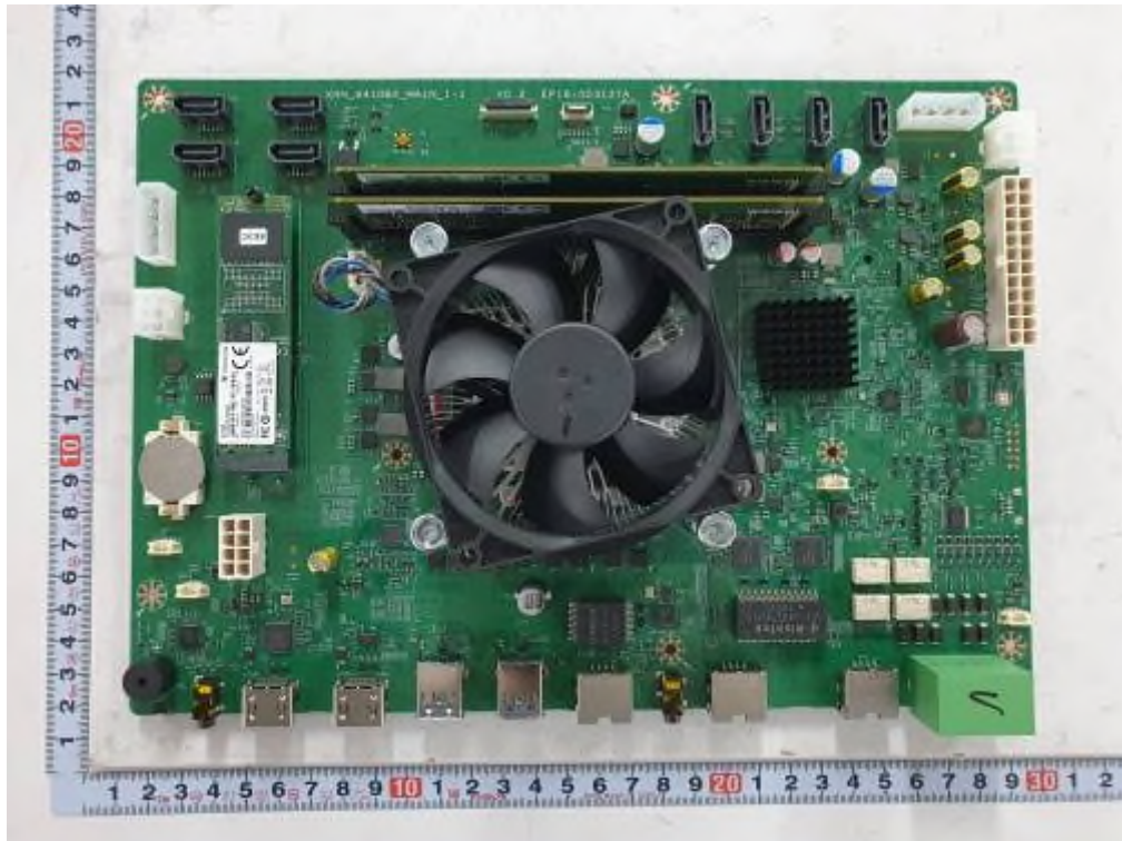
<Photo 16 > Component view (Main board - Non RAID type)
