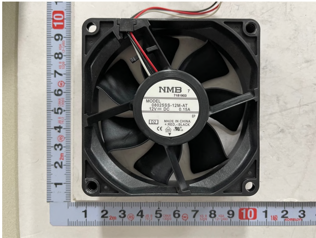
<Photo 23 > DC Fan (near SMPS board)
