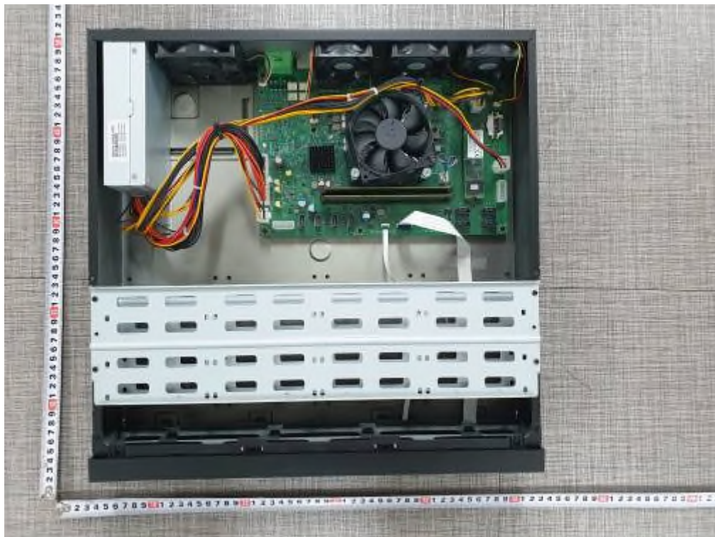
<Photo 8 > Internal view (HDD - Interior mounting type)
