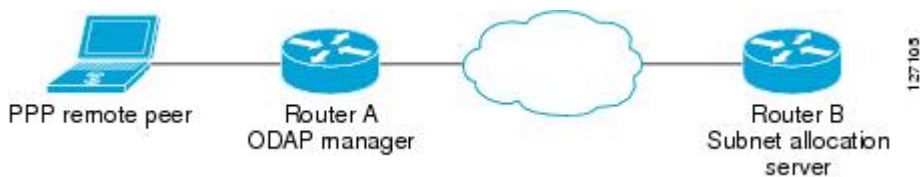
Figure 62: Subnet Allocation Server Topology
