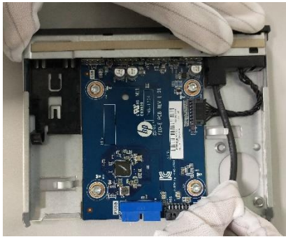
Figure37 Release the front panel mount cable from clip.
