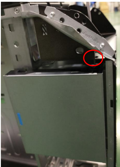
Figure81 Unlock top side screw of ODD bracket cover
