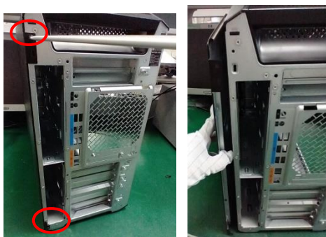
Figure59 Release 2pcs screws of right side panel.
