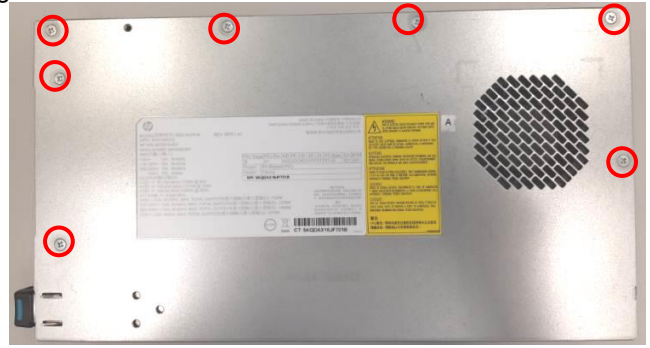
Figure84 Unfasten seven screws.
