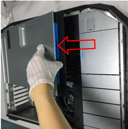
Figure3 Remove the CPU fan duct frame.
