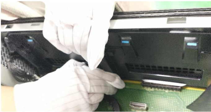
Figure27 Lift the latch and slide to the left (in the direction of rear IO).
