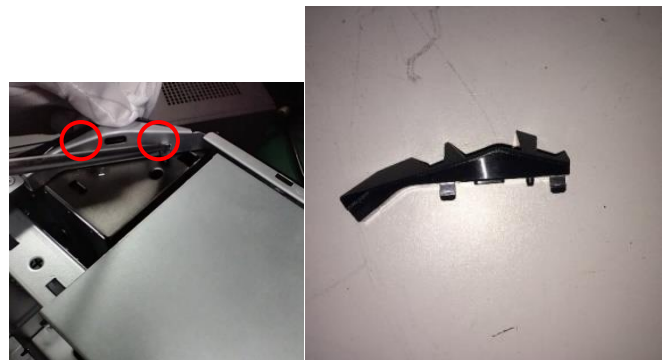
Figure70 Remove the left side plastic parts of corner bracket pocket by release the clasp.
