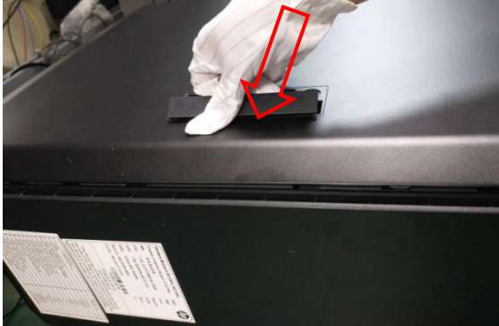
Figure3 Remove the CPU fan duct frame.
