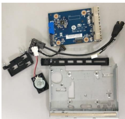
Figure47 Remove ODD housing from chassis.
