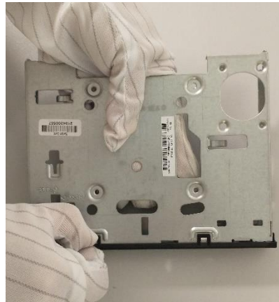
Figure46 Remove the 3pcs HDD brackets from chassis.
