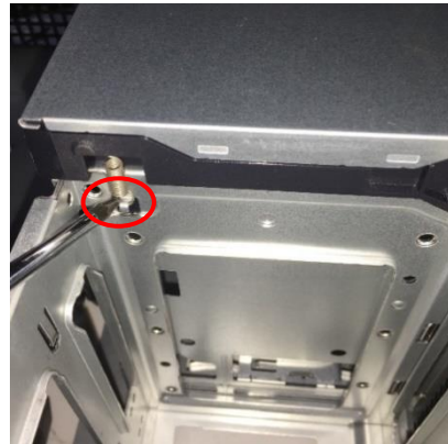
Figure82 Remove the ODD bracket cover
