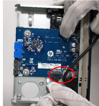
Figure40 Release the front panel mount cable by push out 2 pins fixed black side in switch card tray.
