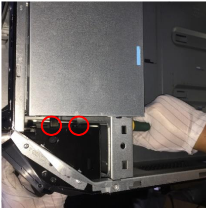
Figure75 Unlock 2pcs screws front side handle.
