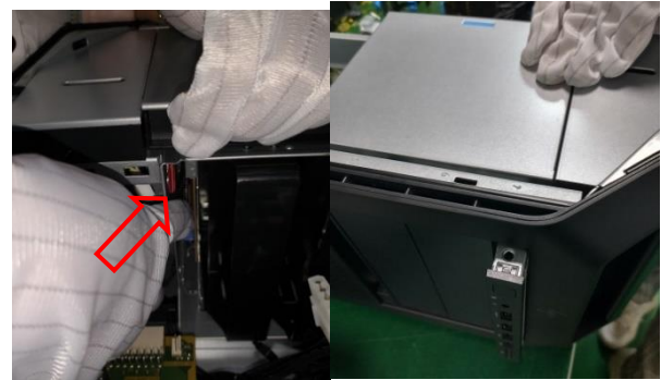
Figure34 Remove the switch card from chassis.
