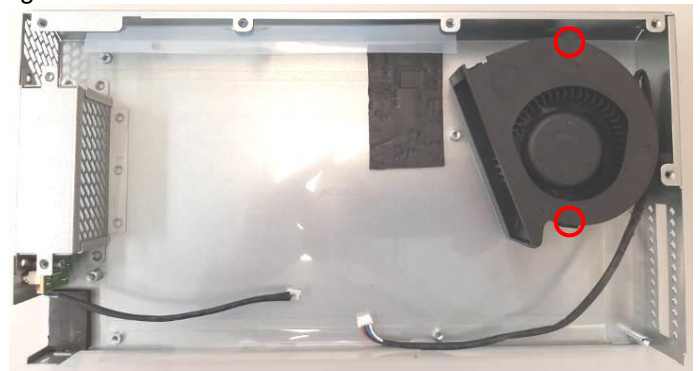
Figure94 Unfasten two screws.
