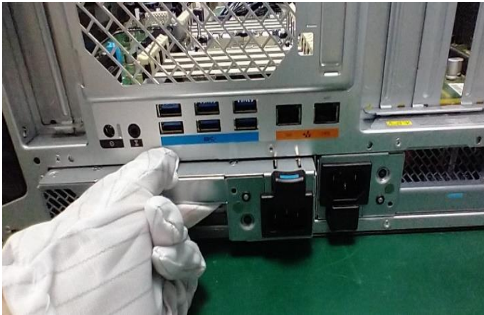
Figure53 Press the bottom and remove the 2pcs PSU.
