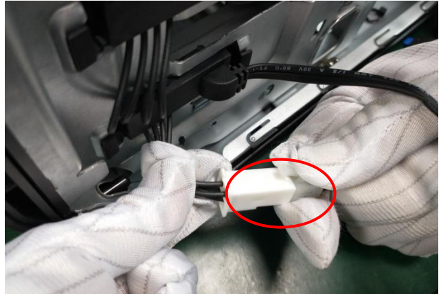
Figure62 Disconnect the H1 power cable and blind mating SATA power cable
