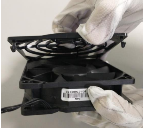
Figure31 Remove the fan guard from fan.
