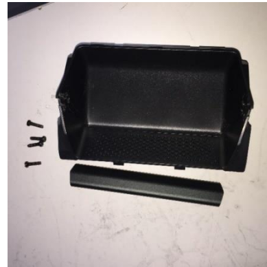
Figure74 Remove the handle pocket and details of front side handle pocket
