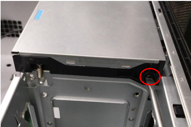
Figure81 Unlock top side screw of ODD bracket cover
