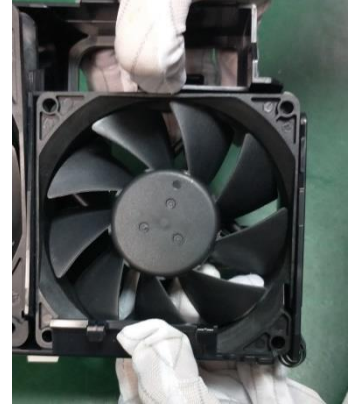
Figure20 Remove the front middle chassis fan from fan guide.
