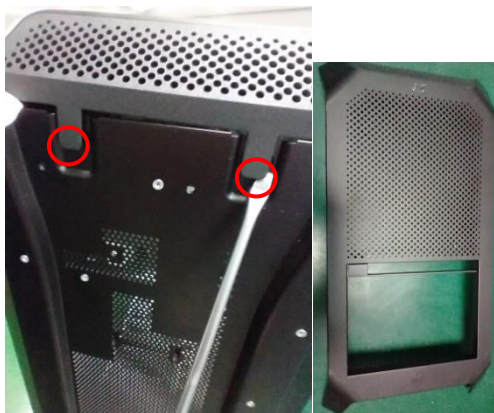
Figure69 Release clasp of front bezel on bottom side of chassis and remove the bezel
