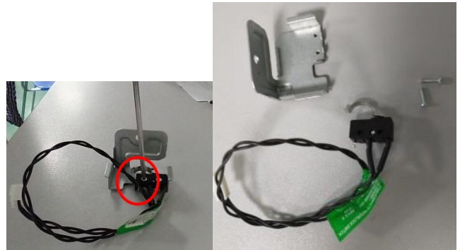
Figure68 Release 2pcs latches of top bezel and remove it.
