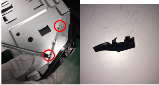
Figure73 Release 2pcs latches of front side handle pocket.
