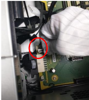
Figure29 Disconnect the front upper chassis fan cable.
