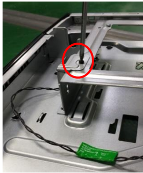
Figure67 Push up 2pcs inside latches to release hood sensor bracket from chassis.
