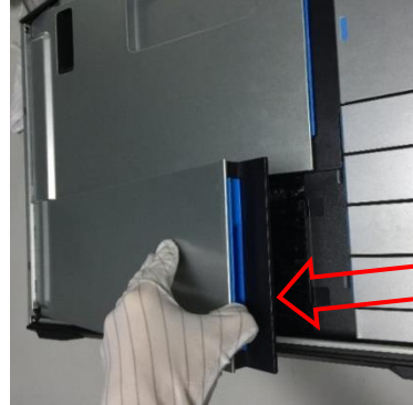
Figure4 Press the latch and push the top PCI card duct out.
