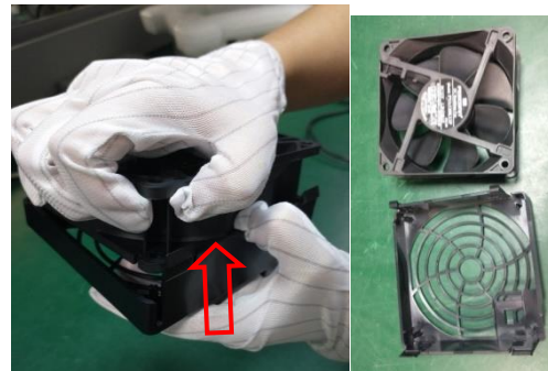
Figure24 Remove the fan guard from fan guard
