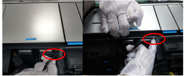
Figure10 Disconnect the ODD SATA/ Power cable from ODD.
