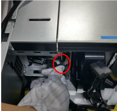
Figure35 Loosen the screws(x2) of speaker and release speaker.
