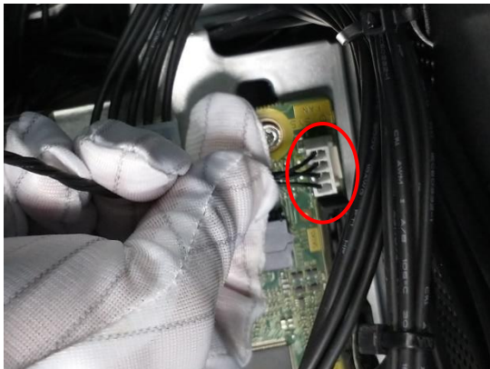
Figure17 Disconnect the front lower chassis fan cable
