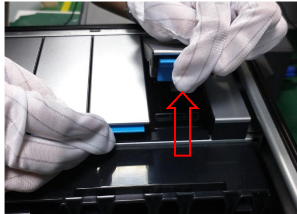
Figure12 Loosen the HDD bracket
