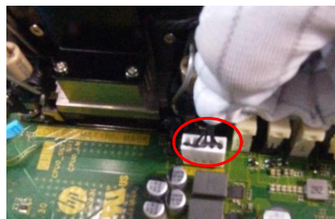
Figure48 Disconnect the CPU cooler cable from Motherboard.
