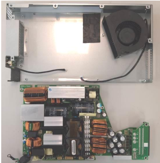
Figure93 Take out PCBA with AC socket cable from bottom chassis.
