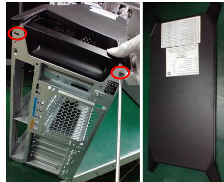
Figure68 Release 2pcs latches of top bezel and remove it.
