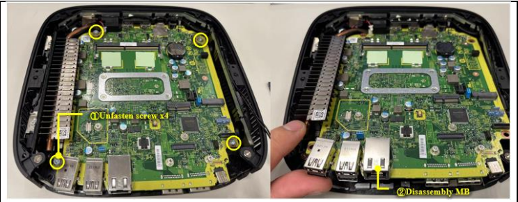
STEP 12. Unfasten "+" M2 screws and internal antenna
