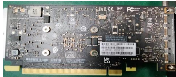
Figure10 Press the button and remove the graphic card from motherboard, See below is Graphic card PCB area >10 sq cm
