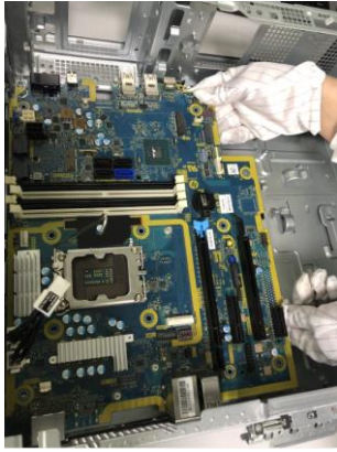
Figure25 Remove the motherboard from chassis.
