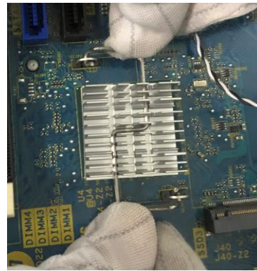
Figure24 Use Philip #0 screwdriver to loose the screws from motherboard.
