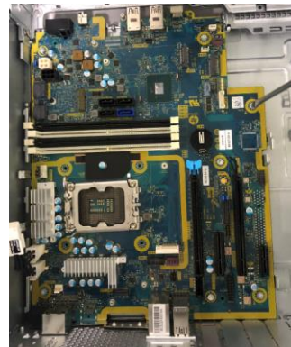
Figure24 Use Philip #0 screwdriver to loose the screws from motherboard.
