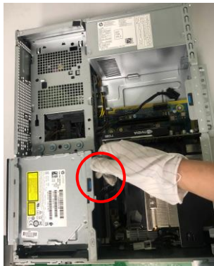
Figure3 Disconnect the ODD SATA/ Power cable from ODD
