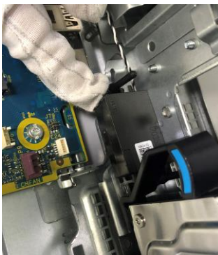
Figure23 Remove speaker from Chassis.
