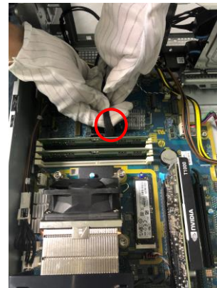
Figure6 Disconnect the SATA cable from Motherboard.
