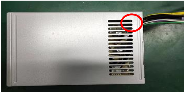
Figure27 Cut the cable tie
