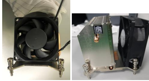
Figure14 Use Philip #0 screwdriver to loose the screws and separate the fan from cooler
