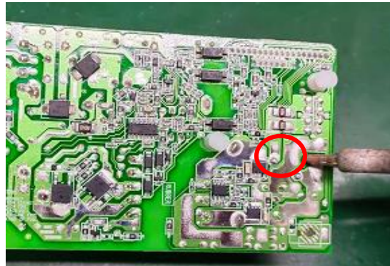
Figure34 Remove capacitors use solder iron.
