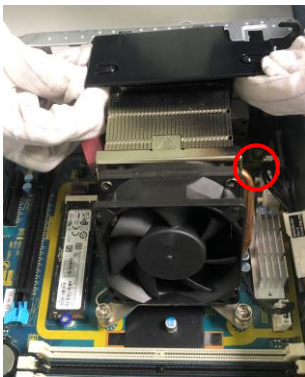
Figure11 Disconnect the cable and remove the fan duct from cooler
