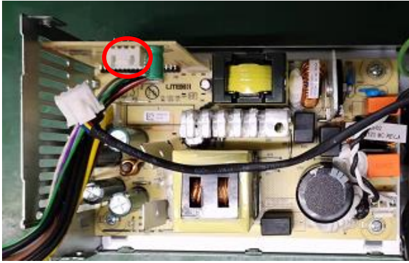
Figure33 Cut output cable, AC inlet wire, LED wire. There are tw PCA with a surface greater than 10 sq cm on PSU.
