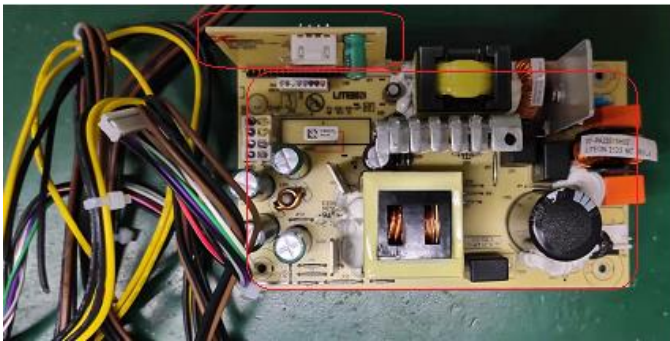
Figure35 Heat the solder of Electrolytic Capacitors greater than 2.5cm in diameter or height and remove it.( C103、 C305、 C306、 C307、 C309)
