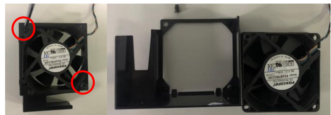
Figure12 Use Philip #0 screwdriver to loose the screws and remove the fan
