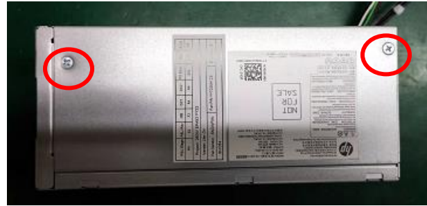
Figure28 Remove screw for top.
