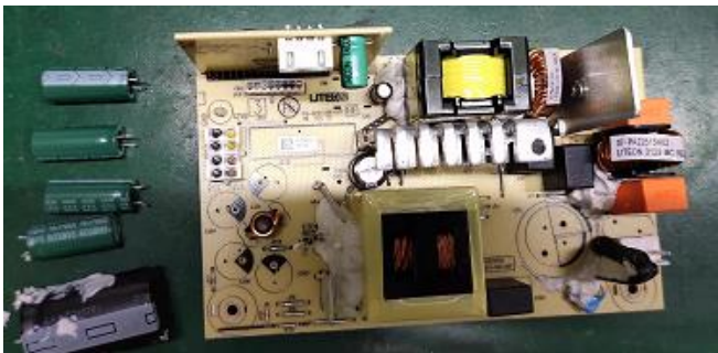
Figure35 Heat the solder of Electrolytic Capacitors greater than 2.5cm in diameter or height and remove it.( C103、 C305、 C306、 C307、 C309)
