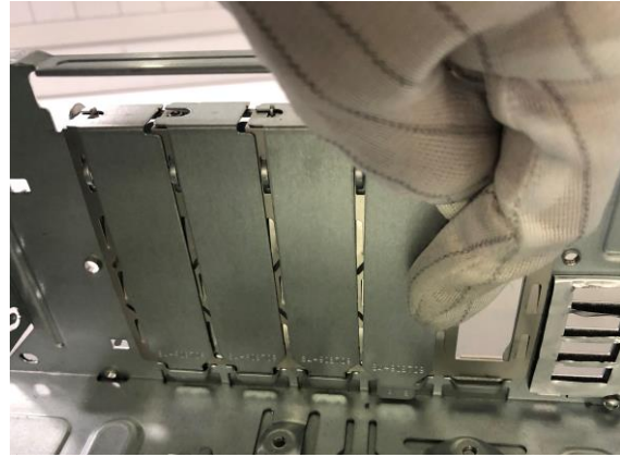
Figure26 Remove the PCI slot covers (x5) from chassis
