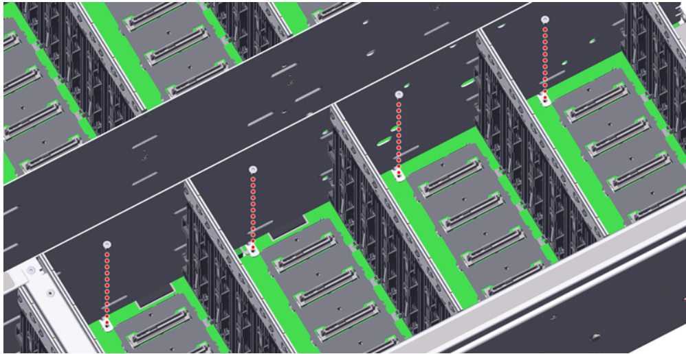
Figure 49: Rear-Right Drive Bays, As Viewed from Right-Front-Top
