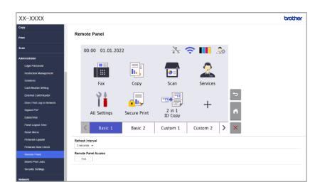
The Brother Remote Panel software solution allows to remotely operate the control panel of a Brother machine from its Web Based Management. The operator can then use it to interact with the machine's LCD and panel buttons to retrieve diagnostic information for troubleshooting purposes. This solution can also be used for training and demonstration purposes.
