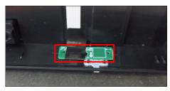
Use a Philips-head screwdriver to remove 4pcs screws for unlocking the bracket chassis with the panel.
