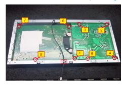
Remove the power board and interface board with S18 TBT Board from the bracket chassis carefully, and then disconnect all of the cables.
