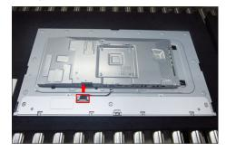
Take away the bracket chassis module and then put S15 the bracket chassis module on a protective cushion.
