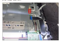
Tear off all tape to release the cables and release sensor board from the hook of the rear cover. Use a Philips-head screwdriver to remove 2pcs screw for unlocking the key board.
