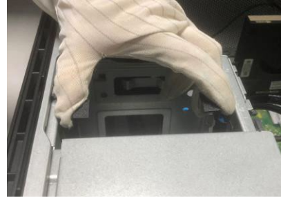
Figure6 Press the HDD's latch on HDD tray, and remove the HDD tray from HDD cage
