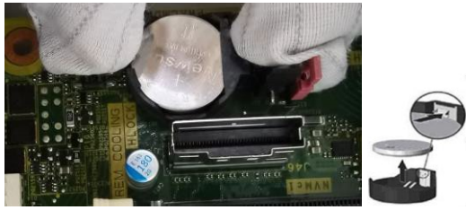
Figure29 Remove the battery from the MB.
