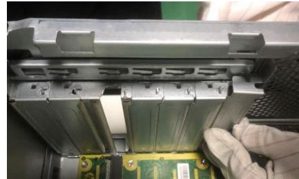
Figure20 Release the PCI snaps.
