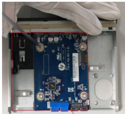
Figure41 Loose the 4pcs switch card PCA screws and remove the switch card PCA. See below PCA area>10 sq cm.
