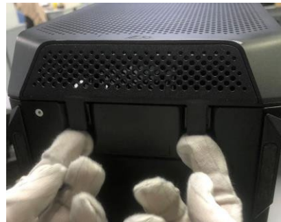
Figure32 Remove the front panel from chassis.
