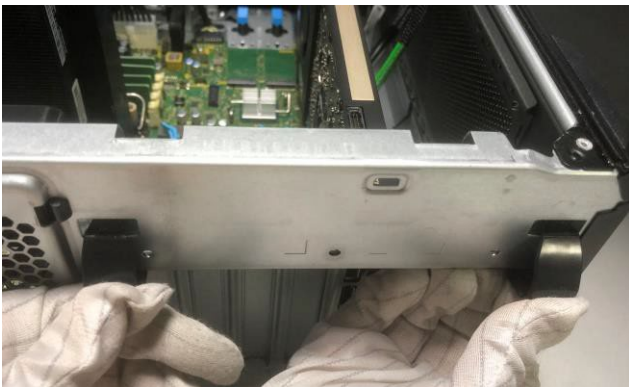
Figure9 Loose the PCIE retainer.
