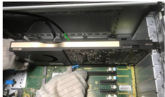
Figure10 Remove the graphic card from MB.
