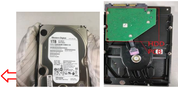
Figure5 Remove the HDD from HDD tray. See below HDD PCB area >10 sq cm.
