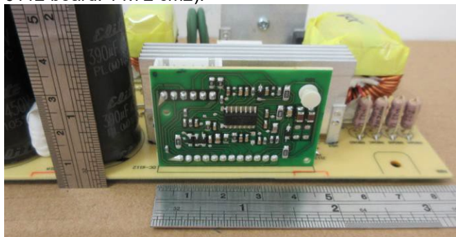
Figure52 Identity PCBA > 10 cm 2 for further treatment (DC-6112 board: 14.72 cm 2 ).
