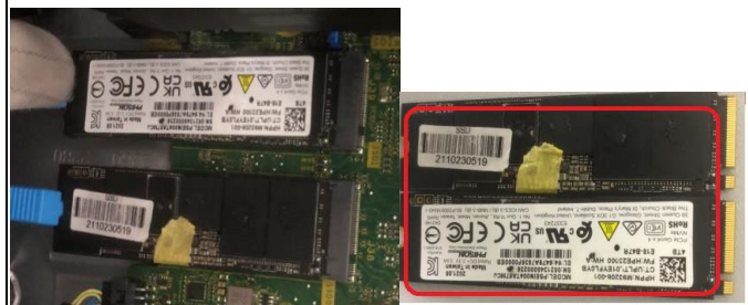
Figure8 Remove the 2pcs SSD. See below SSD PCA area >10 sq cm.
