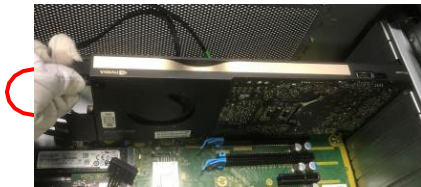
Figure7 Disconnect the cooler cable.
