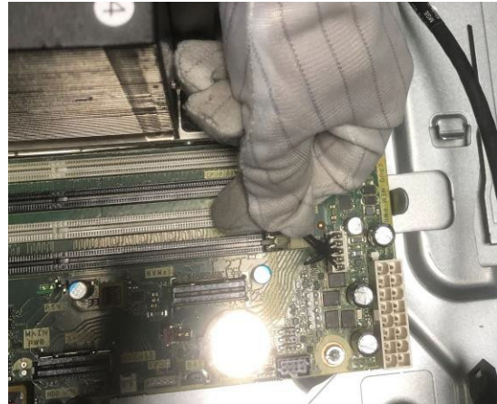
Figure22 Disconnect the cooler cable from MB.
