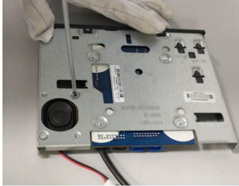
Figure35 Loosen the screws(x2) of speaker and release speaker.
