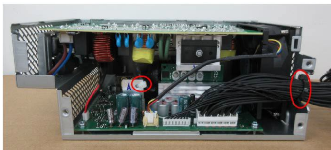
Figure51 Identity PCBA > 10 cm 2 for further treatment (EMI board: 161.2053 cm 2 ).
