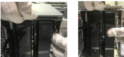
Figure33 Release the latch.
