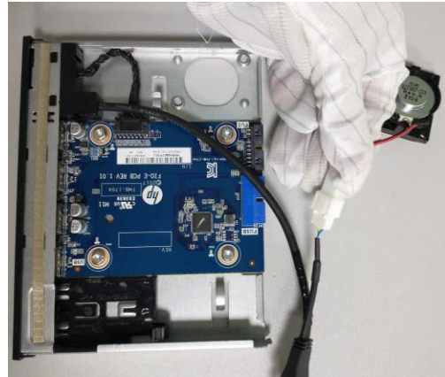
Figure38 Disconnect the front panel mount cable from switch card
