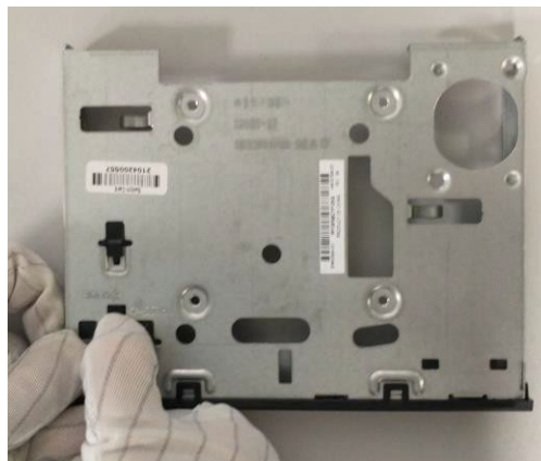
Figure42 Remove the SD card reader carrier.
