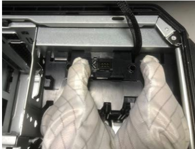
Figure27 Press the 2 latch to Separate the fan from front fan housing.
