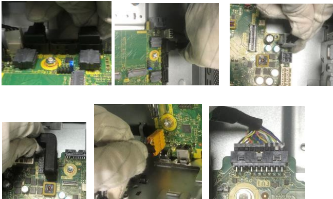
Figure21 Disconnect all other cables from MB.
