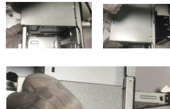
Figure34 Remove the FIO module and ODD devices from cage
