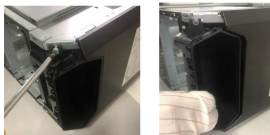
Figure46 Loose the 2 screws to remove the front handle from chassis.
