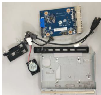
Figure45 Detailed parts of switch card assembly.
