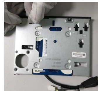
Figure40 Release the front panel mount cable by push out 2 pins fixed black side in switch card tray.
