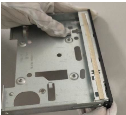
Figure43 Loosen the left and right side hooks of switch card panel.
