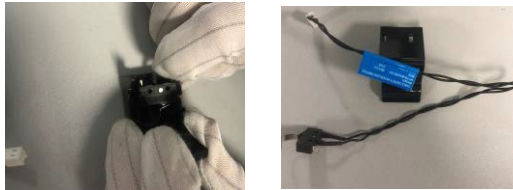
Figure19 Separate interlock holder from cable.
