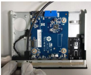
Figure39 Release the front panel mount cable by push out 2 pins fixed front side in switch card tray.
