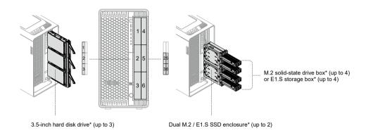
Note: M.2 / E1.S SSD enclosure priority is higher than 3.5-inch hard disk drive.
