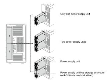
Note: Power supply unit bay storage enclosure priority is higher than power supply unit.
