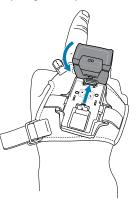
2. Push down on the scanner to snap into place.
