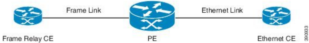
Figure 47: Frame Relay-Ethernet Local Switching Topology
